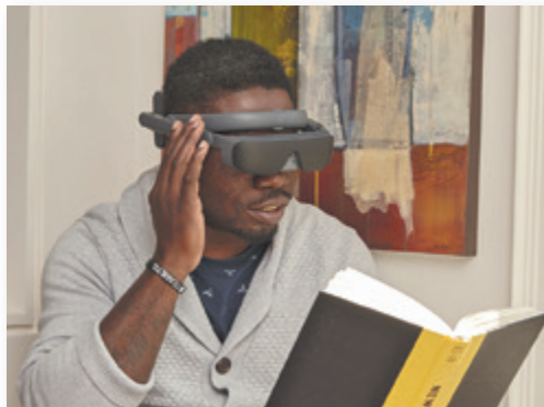
A video display system captures what it sees and projects images onto screens in a headset.
